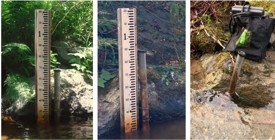
Figure 18. Cook Creek logger housing in May 2019 (Left), July 2022 (Center), and February 2023 after loss of staff gauge (Right).
