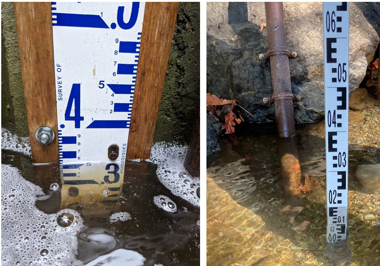
Figure 5. A typical staff gauge , displaying a stage of approximately 0.355 m (Left). Reference point reading using a portable stadia rod placed on a submerged benchmark , displaying a stage of approximately 0.200 m (Right).
