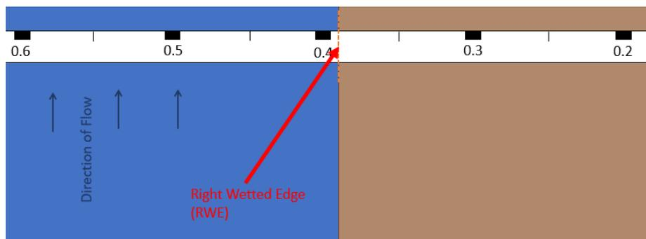
Figure 7. How to determine the wetted edge.
