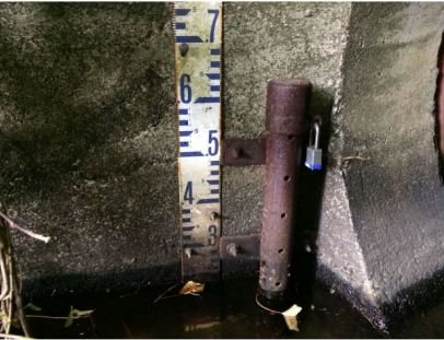
Figure 1 - Photo of reference gauge used during operations from 2012 to 2022. Staff gauge is assumed to be stable and a gauge correction of 0.000m applied.
